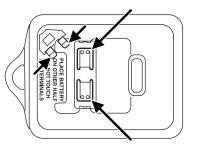
orientation of the battery. Press the battery down to ensure that the battery is fully seated in the battery housing cavity.
